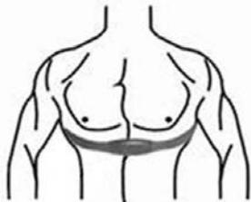
The sensor in the chest belt transmits the heart rate direct to the computer. The maximum range of the sensor is 85 cm. If the sensor is more than 85 cm removed from the computer, the signal will be too weak to be received. Clean and dry the chest belt after use. If this is not done properly, the sensor may remain switched on, as it senses moist or perspiration, resulting in empty batteries.
